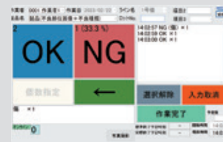
Real-time collection and calculation of work time and inspection results
